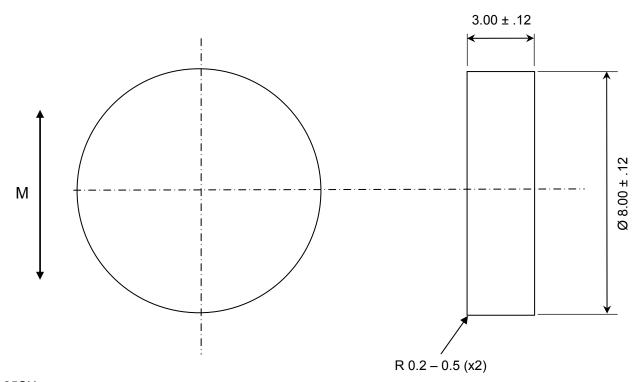
$X.XX = \pm .01$   $X.X = \pm .25$   $X.XXX = \pm .005$   $X.XX = \pm .13$   $\frac{ANGLES}{\pm .5^{\circ}}$  DO NOT SCALE DRAWING
